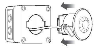
Pull out spring tab and rotate spring arm as shown, then insert into enclosure aperture. Finally rotate MSensor body for location.
