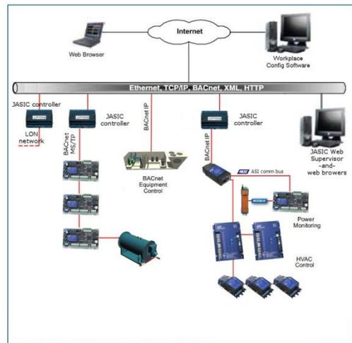
Figure 1: An overview of the Tridium architecture in a building.
